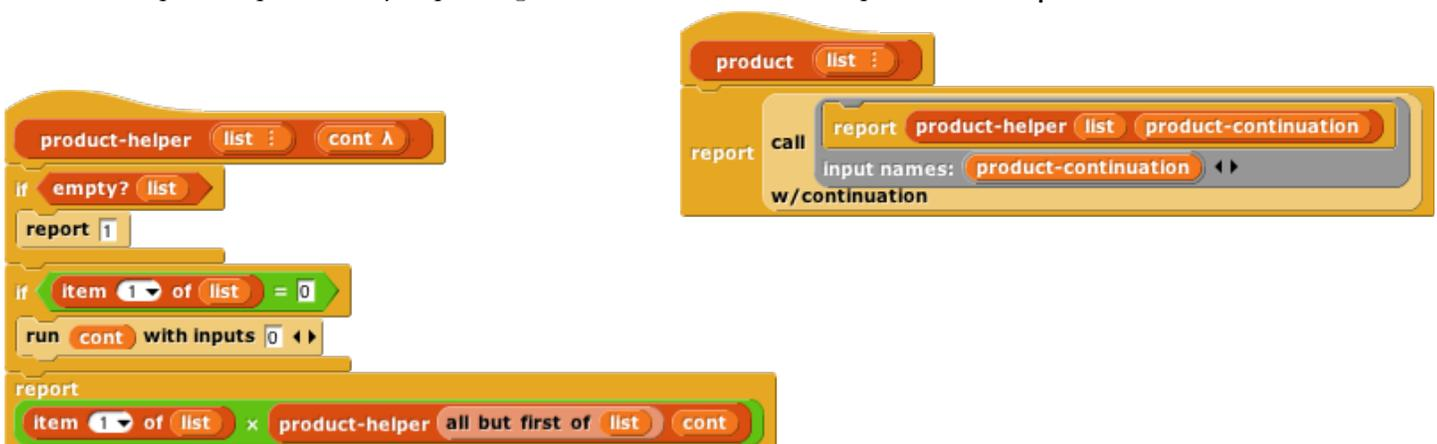
The `call w/continuation` block takes as its input a one-input script, as shown in the **product** example. It calls that script with *the continuation of the call-with-continuation block itself* as its input. In this case, that continuation is
